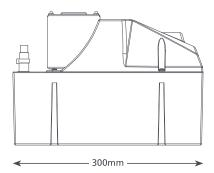
**HOT WATER ECONOMY @ 230 VAC 50Hz** Max. flow 900L/h @ 0m head Max. rec. head 6m Tank capacity 4L dB(A) @ 1m 60 Power supply 230 VAC, 1.5A, 50Hz Rated Non continuous Class I appliance 1200kW / 4m Btu/h Max. unit output Max. water temp 100°C / 212°F Inlet/outlet size x2 40mm in, 10mm out IP Protection IP20 Safety switch 3.0A Normally closed Thermal protection Fully potted n/a
