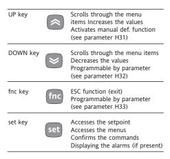
At start-up the instrument performs a Lamp Test; for few seconds the display and the leds blink, in order to verify their integrity and correct operation. The instrument has two main menus: the "Machine Status" and "Programming" menu.
