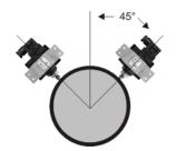
**Figure 3: Mounting Position Range**
